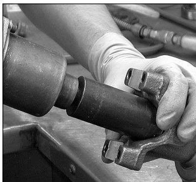
1/2" impact gun on pinion nut
