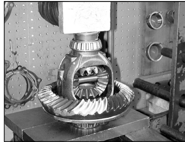
Pressing on carrier bearing
