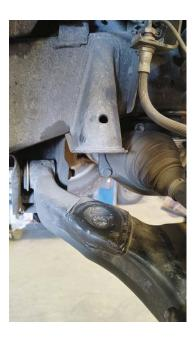
**4.** Using the access hole on the opposite side of the bracket, install the new Superbump bump stop with the provided special hex wrench and a 14mm wrench. Repeat steps 1-4 on the opposite side of the truck.
