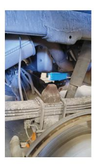
2. Loosen U-bolts enough to remove the factory bump stop.
