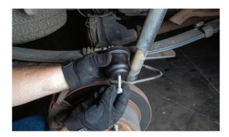
**3.** Using the provided 8mm Allen wrench install the Superbump and mounting bolt into the stock bump stop location.
