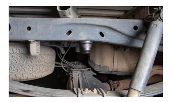
**1.** Using a 13mm socket, remove the stock bump stop mounting bolt and stock bump stock.
