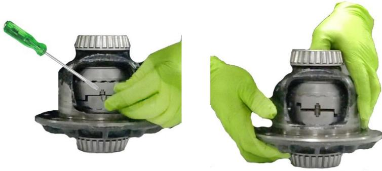
**NOTE:** The springs are firm. Place the spring in the bottom of the pocket, then use a small flat head screwdriver to compress the spring and pop it into the top pocket.
