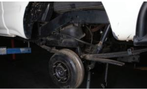
**STEP 3**Loosen nuts and remove u-bolts with appropriate socket.
