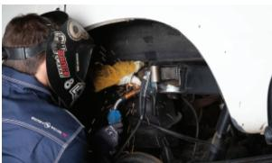
**STEP 8**Check alignment of the new bracket. It is suggested to reinstall the wheels and let the vehicle down. This is to ensure proper fit before final welding.
