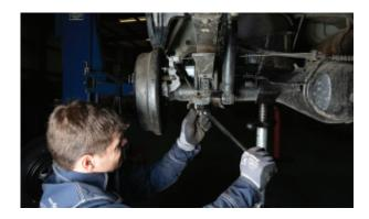
**STEP 6**Use the grinder with the cut off wheel and flap wheel to cut off the stock striker pad on the frame of the truck.
