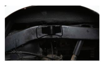
**STEP 11**Install bump into bracket and tighten to desired height with included spanner wrench.
