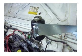
Mount the reservoir to the bracket as shown. Be sure the curve of the bracket is facing downward.
