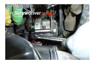
Tension the V-Belt by prying the alternator away from the engine and tightening the adjustment bolt.
