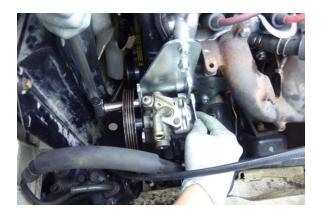
While holding the pivot bolt with a 12 mm box end wrench, snug the nut with a 12 mm deep socket.
