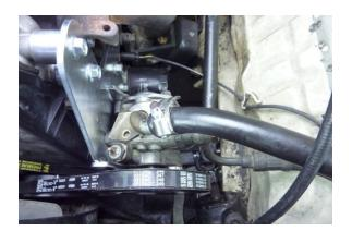
Connect the supplied (5/8") pump-toreservoir hose to the pump and tighten the clamp.
