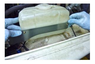
Align the bracket with the holes in the washer fluid reservoir and insert the supplied (M6-1.0 X 16) bolts as shown.
