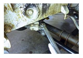
LOOSEN the castle nut (4 or 5 turns) using a 17 mm box end wrench.
