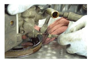
Disconnect the electrical connector if equipped.
