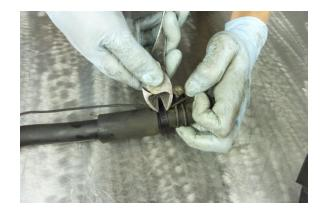
Loosen the hose clamp on the pump-toreservoir hose using a 7 mm socket (or phillips screwdriver) and disconnect the hose. Set the reservoir aside.
