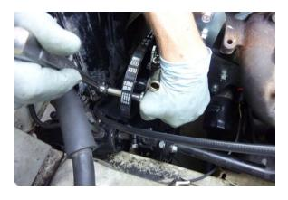
Tension the belt by lifting up on the pump and tightening the adjustment bolt using a 12 mm deep socket. 7.5 to 11.5 ft. lbs.
