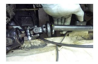
To shorten the steering shaft, place the spline end on a board and hit the rag joint end with a hammer. You have to hit pretty hard to start the collapse, but once it starts, in goes pretty easy. Try not to over collapse (shorten) the shaft. It is easier to collapse than to lengthen. As you get closer to the correct length, test fit the shaft and continue adjusting until it fits properly.
