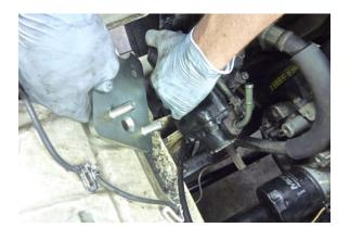
Shift the steering gear toward the passenger side of the vehicle and position the supplied pump bracket between the steering gear and the frame.
