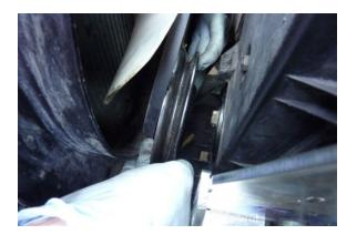
Remove the crankshaft pulley.
