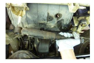
Disconnect the other end of the steering damper by removing the damper-to-frame nut and washer.
