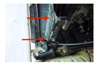
Remove the two driver side radiator bracket bolts using a 10 mm socket.
