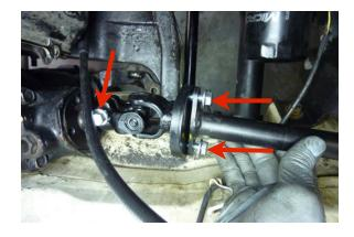
Double check to see that the pitman arm is still parallel with the frame and the steering wheel is still centered. If they are not, repeat **Steps 66 through 71.** If all is still aligned properly, continue to the next step.
