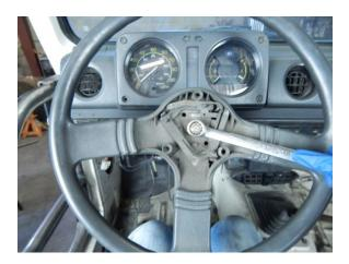
Step 44 Snug the nut and then torque it to 20 ft. lbs.
