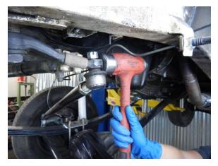
Strike the end of the pitman arm sharply until the drag link tapered stud comes loose form the pitman arm.
