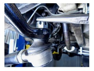
Step 35 Bend the upper (long) leg up and over the top of the top of the tapered stud.
