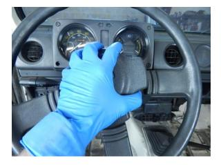
Step 39 Remove the horn button by pulling it upward.
