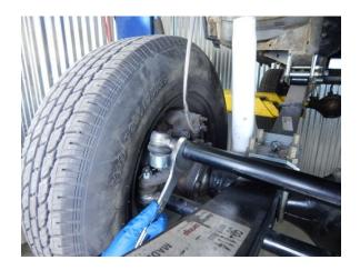
Step 28 Loosen the passenger side drag link jam nut.
