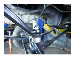
If the cotter pin holes do not align, TIGHTEN (never loosen) the castle nut until the cotter pin holes do align.
