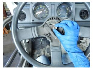
Step 43 Reinstall the washer and nut.
