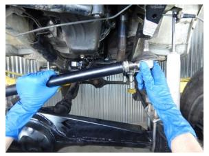
Hold the drag link end with your right hand and rotate the drag link adjusting sleeve with your left hand until the tapered stud will fit into the pitman arm.
