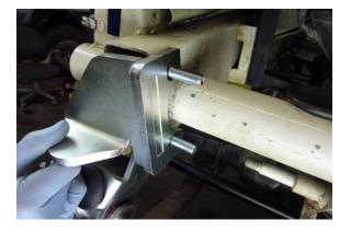
Step 38 Install the bump stop on the bolts as shown.
