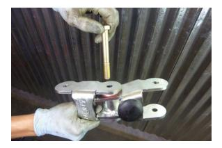
Force the upper link and the lower link together and install the supplied (1/2X20X4") bolt.
