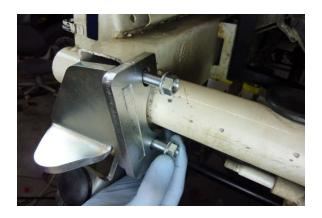
Step 39 Install the (2) serrated nuts and torque them to 25 ft. lbs.
