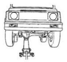
**Tech Tip** Proper positioning of floor jack.
