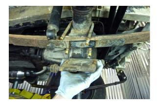
Step 8 Remove the U-bolt plate.
