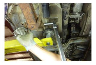
Step 32 Tighten the passenger side hanger nut 43 to 61 ft. lbs.
