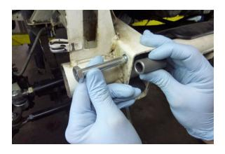
Step 37 Install the supplied upper bolt (M10X1.25X80) and the spacer sleeve as shown.
