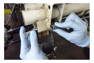
Step 36 Beginning on the passenger side, install the supplied lower bolt (M10X1.25X80) and the spacer sleeve as shown.
