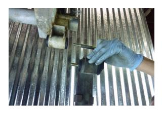
Step 16 Remove the shackle and leaf spring and set this assembly aside.
