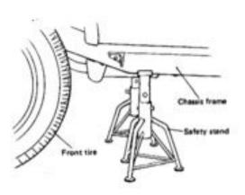
Tech Tip Proper positioning of safety stands.
