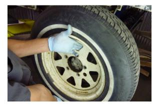
Install both front wheels and torque the lug nuts 36 to 57 ft. lbs.
