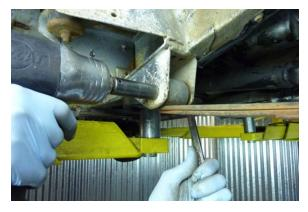
Remove the spring mount bolt using a 17 mm socket and 17 mm combination wrench.
