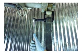
Step 14 Remove both shackle nuts using a 14 mm socket.
