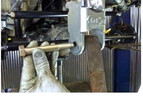
Position the "Rear" leaf spring in the lower link and install the supplied (1/2X20X4") bolt.
