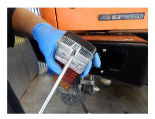
Step 57 Ready the tail light for installation by removing the (2) phillips screws using a phillips screwdriver.
