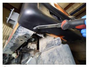
Step 6 Remove the bottom retainer button using an upholstery tool.
