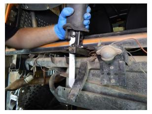
Step 24 Cut the center bumper bracket flush with the body.
