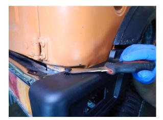
Step 5 Remove the top retainer button using an upholstery tool.
