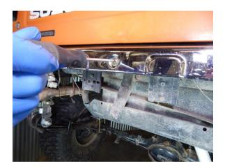
Step 14 Remove the center mounting screw using a #3 phillips screwdriver.
