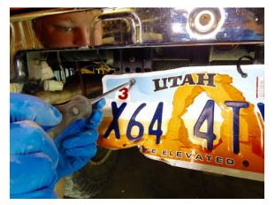
Step 9 Remove the license plate using a phillips screwdriver.
