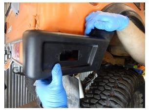
Step 7 Remove the bumper corner by snapping it loose at the top and bottom.
