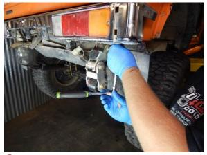
Step 12 Remove the 2 passenger side, outside bumper bracket bolts using a 10mm socket. (See next picture)
