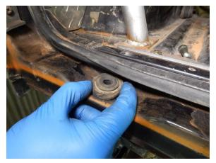
Step 19 Remove the rubber bushing.
