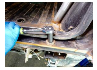
Step 20 Remove the passenger side body mount bolt, washer and rubber bushing.
