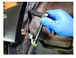
Step 4 Remove the (2) fender flare bolts using a 10mm socket.
