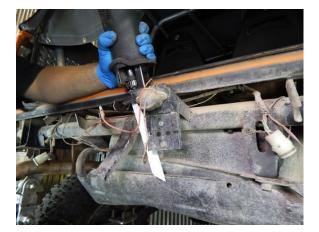
Step 25 Cut off the passenger side license plate light bracket.
