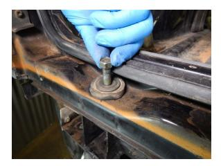
Step 18 Remove the body mount bolt and flat washer.
