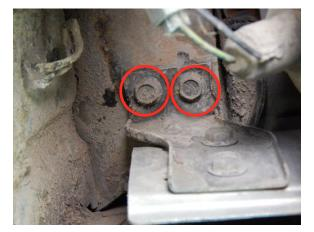
Tech Tip 12 These are the passenger side, outside bumper bracket bolts.
