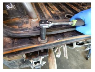
Step 17 Loosen the driver side body mount bolt using a 14mm socket.
