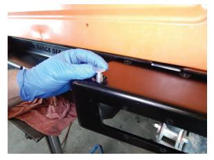
Step 48 Install the passenger side bumper wing following the same steps shown on the driver side bumper wing. Steps 43 through 47.
