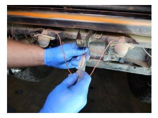
Step 21 Unplug the (2) license plate light electrical wires.
