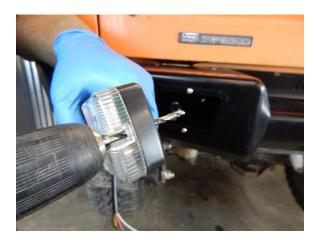
Step 58 Drill out both holes using the supplied 13/64" drill bit.
