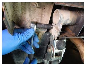
Step 27 Remove the driver side brace plate if it is still present using a 10mm socket.
