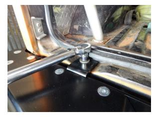
Step 54 Torque the (2) body mount bolts to 25 ft. lbs.
