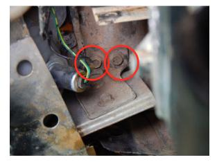
Step 13 Remove the driver side, outside bracket mounting bolts using a 10mm socket.
