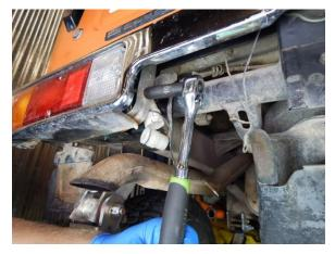
Step 10 Remove the driver side, inside bumper bracket bolt using a 10 mm socket.
