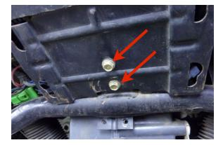
Remove the radio bracket by removing the (2) bolts using a 10 mm socket.
