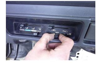
Step 4 Pull off the (4) heater control knobs.
