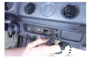
Work the climate control assembly back into position and install the (2) mounting screws.
