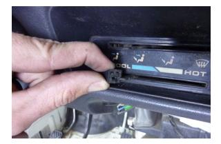
Step 18 Install the (4) control lever knobs.
