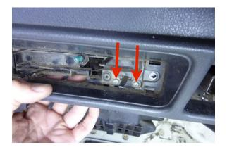
Step 9 Remove the (2) blower switch mounting screws.
