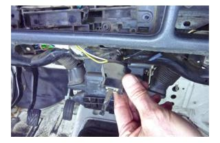
Remove the blower switch from the bottom of the climate control assembly.
