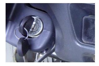
Turn the ignition switch to the on position and check the fan motor in all speeds.
