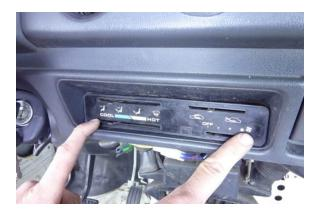
Step 17 Position the faceplate over the control levers and snap it into place.
