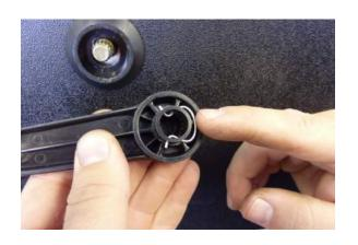
**Tech Tip**Correct positioning of window handle clip.
