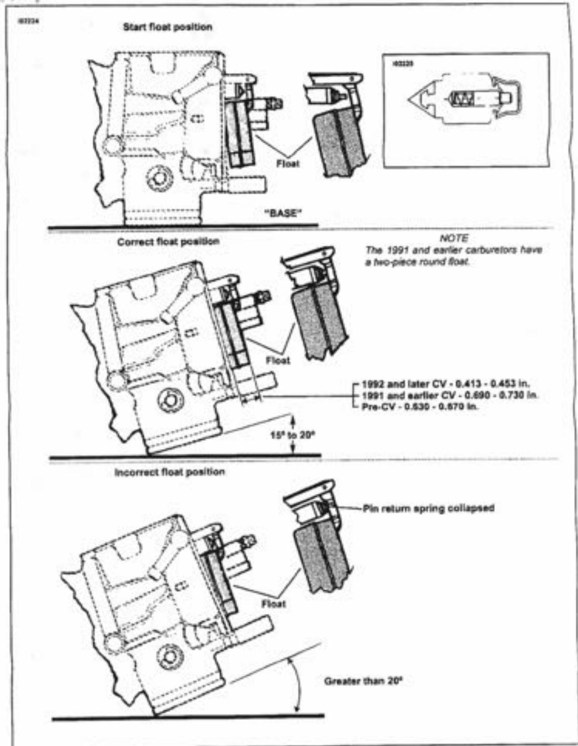
Figure 1. Float adjustment
