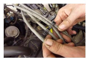
Step 2 Disconnect #1 spark plug wire from the harness connector.
