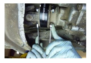
Step 10 Tighten the nuts 17.0 to 21.5 ft. lbs.
