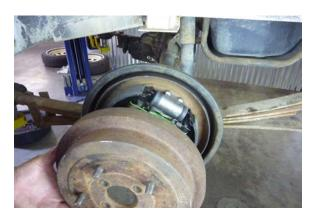
Step 41 Install the brake drum.
