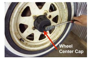
Remove the wheel center cap by removing the (1) center bolt using a 14 mm socket.
