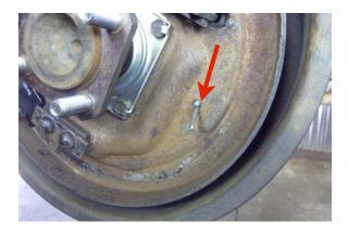
Step 34 Install the rear shoe hold down pin from the rear of the backing plate.
