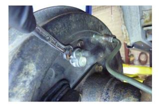
Position the new wheel cylinder as shown.
