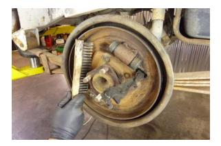
Step 20 Clean the backing plate with a wire brush.
