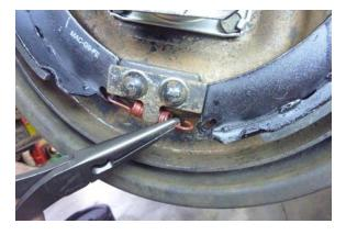
Step 37 Install the return spring B.
