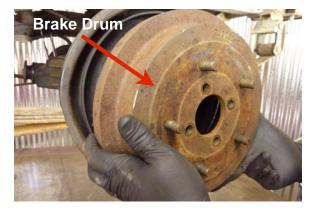
Step 8 Remove the brake drum and set it aside.
