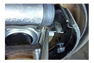
Step 38 Install the rod spring.
