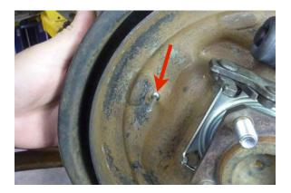
Step 31 Install the forward shoe hold down pin from the rear of the backing plate.
