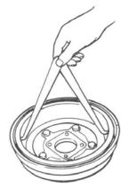
Also inspect the drum for excessive wear by measuring the inside diameter of the drum. If the drum measures greater than 8.740" it will need to be replaced.
