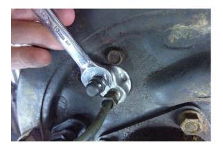
Reinstall and tighten the brake bleeder screw.
