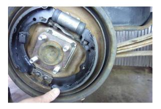
Step 35 Position the rear brake shoe as shown.
