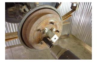
Install the center cap bracket and axle hub nuts and torque. (36 to 57.5 ft. lbs.)
