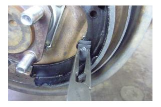
Depress the brake shoe hold down spring, twist the hold down pin 1/4 turn and then release the spring.
