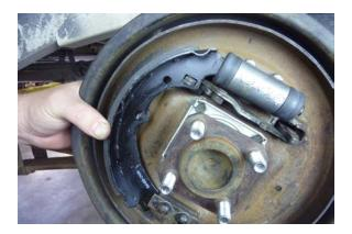
Position the forward brake shoe as shown.
