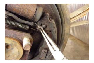
Step 15 Remove the rod spring.
