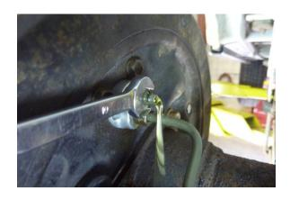
Bleed the brake system according Suzuki Service Instructions.
