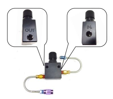
Set up the rest of the proportioning valve assembly as shown here. Leave all these fittings loose for now and set this assembly aside.
