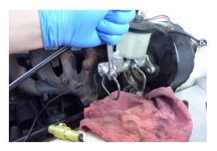
Disconnect the front brake line using a 10 mm tubing wrench.
