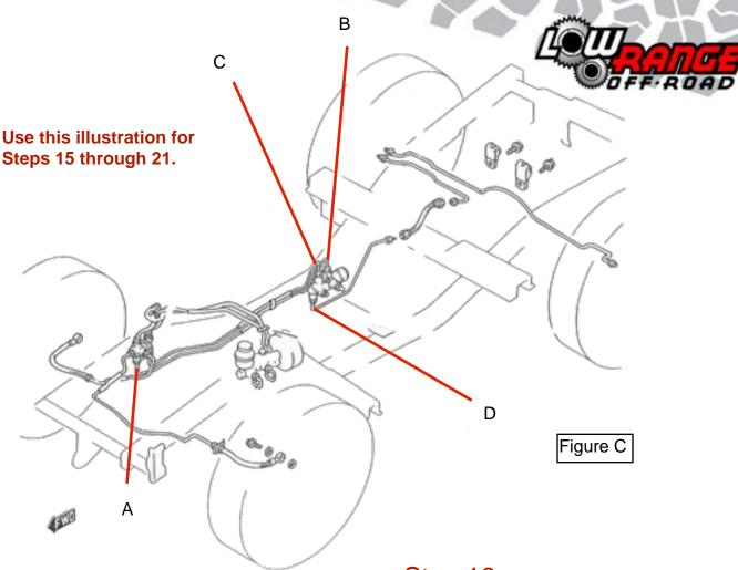
Disconnect the bypass brake line at Point A using a 10 mm tubing wrench.
