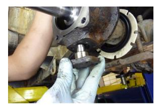
Install the bottom king pin and king pin shim.
