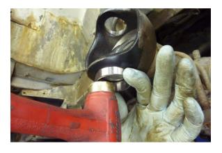
Remove and replace the lower king pin bearing race by repeating **Steps 46 and 47.**
