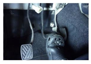
Pump the brake pedal 3 or 4 times to insure the brakes are operating correctly before moving this vehicle. After pumping the pedal 3 or 4 times, the pedal should become hard to push at about 1/2 the distance to the floor. If it does not feel right, seek professional help before driving this vehicle.
