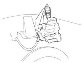
Rest the caliper assembly on the leaf spring or suspend it using a wire.
