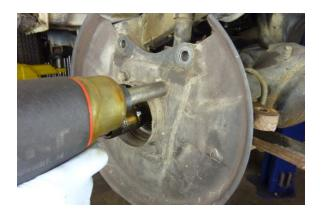
Remove the dust shield, spindle and caliper holder by removing the (4) bolts using a 12 mm socket.
