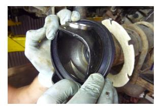
Place the new knuckle ball seal over the knuckle ball.
