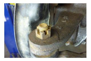
If the slot in the nut does not align with the hole in the stud, as shown here, continue tightening the nut until the hole aligns. Then install the cotter pin and bend one leg as shown in the previous step.
