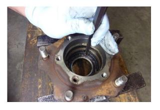
Position two blocks of steel or wood under the wheel studs and drive the inner bearing and hub oil seal out of the hub using a punch and hammer.
