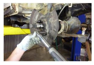
Install the dust shield and hub assembly.
