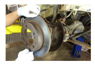
Strike the disc with a ball peen hammer in several locations around the disc as shown. If the disc does not come loose, tighten the bolts a little more and strike the disc with the hammer again. Continue alternating between striking and tightening until the disc comes free.
