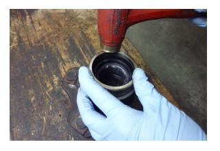
Drive the seal evenly into the hub. Continue driving until the seal is flush with the hub.
