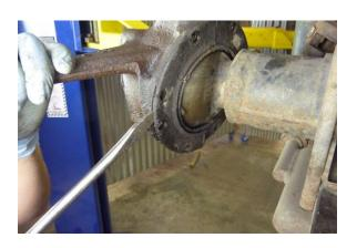
Step 33 Pry loose the oil seal cover halves (front and rear) using a standard screwdriver.
