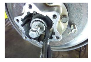
While holding the hub with a larger screwdriver snug these bolts up evenly, in a criss-cross pattern. Then torque them 15 to 22 ft. lbs.
