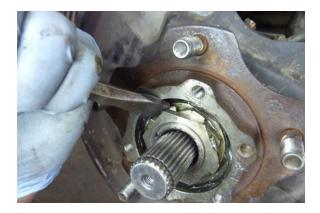
Locate another tab that aligns with one of the flats on the adjustment nut and bend it backward, locking the adjustment nut in place.
