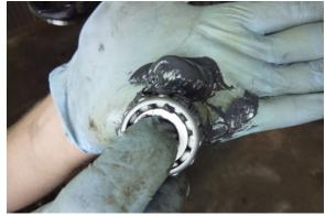
Pack both king pin bearings (upper and lower) with grease. This is done by placing a golf ball size amount of grease in the palm of the hand and holding the bearing with the thumb and forefinger, force small amounts of grease into the bottom of the bearing until it appears at the top.
