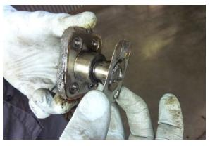
**Tech Tip** If there are shims under the king pins, they must be reinstalled in the same locations. Be sure to mark them or set them aside so you will know where they are to be placed during reassembly.
