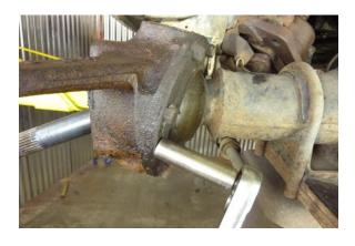
Step 32 Remove the (6) oil seal cover bolts using a 12 mm socket.
