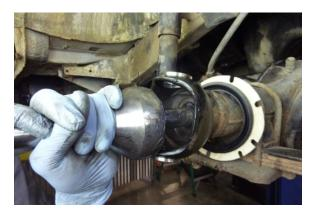
Install the axle in the axle housing until it It will stop when it hits the stops. differential. To install the inner end of in the axle, you will need to push down on the birfield end of the axle, which will lift up on the differential end of the axle, aligning it with the differential side gear. You may also need to rotate the axle slightly, while pushing it in, to align the splines.
