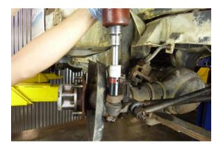
Loosen the castle nut using a 17 mm socket.
