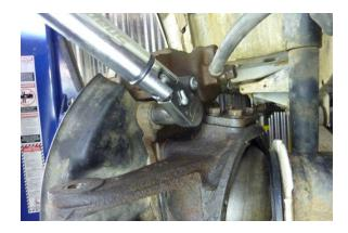
Step 114 Install the caliper adapter bolts and torque them 29 to 43 ft. lbs.
