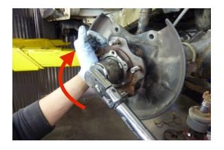
While rotating the hub by hand, torque the adjustment nut to 57 ft. lbs. (8.0 kgm). Back off the nut until torque becomes 0. Then tighten the nut to 7.5 to 10.5 ft. lbs.
