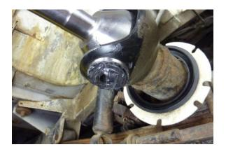
Install the bottom king pin bearing in the bottom race.
