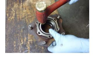
Place the race driver, thin side down, and finish driving in the new bearing race. Be sure it goes in all the way, until it seats against the shoulder inside the hub.
