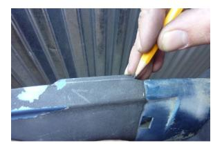
Mark the front of the rear fender flare as shown. This part of the fender flare will need to be trimmed away to accommodate the newly installed rock guard.
