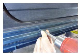
Center punch a mark in the center of each spot weld. This helps center the spot weld drill when drilling.
