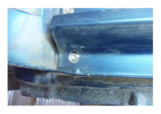
Continue Steps 9 and 10 on all the rest of the spot welds working from the rear of the vehicle forward.
