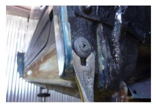
Begin removing the front fender flare by removing the (6) flare clips.
