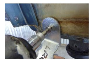
With the screw inserted through the jack nut tool, insert the 4 mm allen socket as shown.
