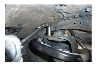
Remove the (3) upper shock mount nuts using 14 mm socket.
