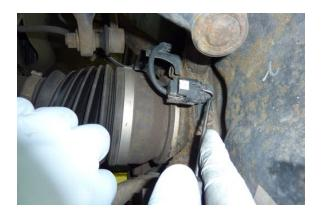
Disconnect the wheel speed sensor using a hook shaped pick tool.
