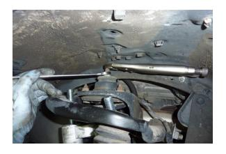
While holding the upper shock absorber shaft with vice grip pliers, remove the upper shock absorber nut using a 17 mm open end wrench.
