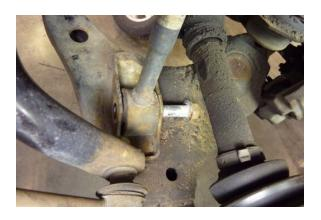
You my have to push down on the lower control arm and brake assembly to free this bolt.
