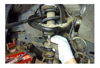
While prying downward on the upper control arm with a larger pry bar, guide the upper ball joint stud into the steering knuckle.
