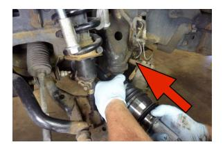
Pop the inboard joint into place with a sharp lunging motion.
