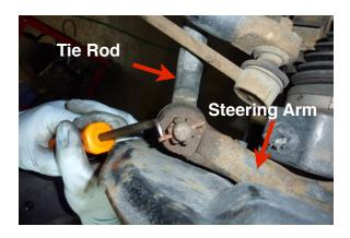
Remove the tie rod end cotter pin using a cotter pin hook tool.
