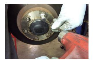
Gently tap the hub cover into place using a small cold chisel and a hammer.
