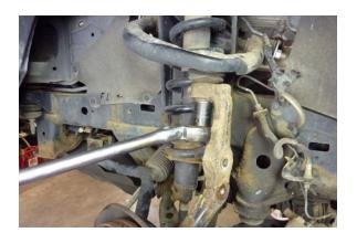
Remove the upper ball joint castle nut using a 19 mm socket.
