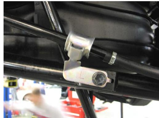
*Correct positioning of the park brake cable.*
