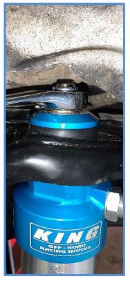
Important Note: The rubber bushings on your King shocks are different from each other. Make sure the taller bushing with the raised center section is on the bottom next to the body of the shock as shown.
