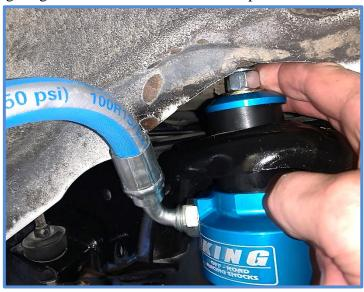
5. Place the rod end on the lower mounting stud and install the factory bolt. Torque bolts to factory specs.
