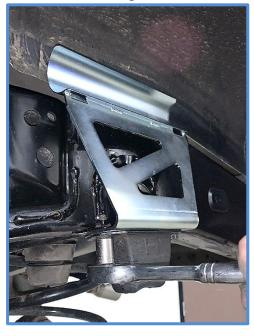
3. <u>Install King Shocks</u> - Shocks are side specific, be sure you are installing shocks on the proper side. (See final install pictures for reference). Start by removing the nut, washer, anodized blue retainer and upper rubber bushing from the upper mounting stud. Make sure the taller bushing is on the bottom of the stud and insert the shock into the upper mount on the vehicle.
