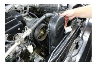
Remove the timing belt cover by removing (8) 10 mm bolts and (1) 10 mm nut.
