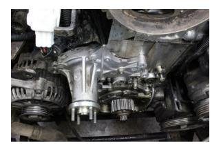
Remove the water pump by removing (2) 10 mm nuts and (4) 10 mm bolts.
