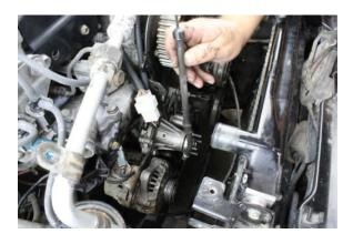
Install the oil dipstick tube and attaching bolt. Don't forget the o-ring.
