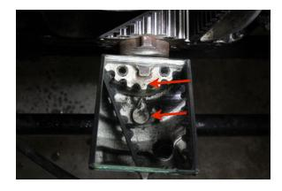
Crankshaft timing marks shown with a mirror. Pulley appears up-sidedown.
