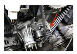
Step 16 Loosen the 10 mm tension lever stud.
