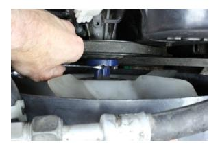
Loosen the (4) 10 mm fan bolts as shown. Do not remove them yet.
