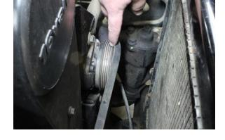
Remove the shroud by removing (2) 10 mm bolts.
