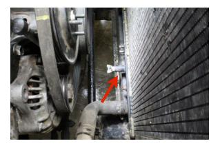
Drain the coolant by opening the drain valve. Turn the valve counter clockwise. Catch the coolant in a clean drain pan so it can be reused or recycled.
