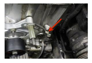
Remove the tensioner lever spring.
