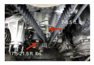
Tighten the tensioner lever stud to 7-8.5 ft. lbs. and the tensioner pulley bolt to 17.5-21.5 ft. lbs.
