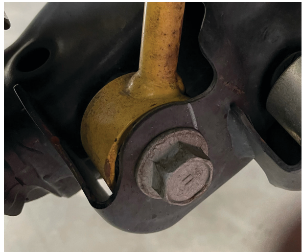
Fig. 5: Remove bolt on lower shock mount.
