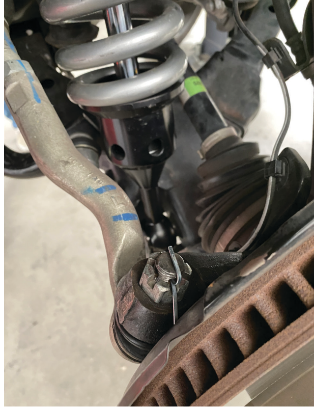
Fig. 10: Reinstall the tie rod end link.
