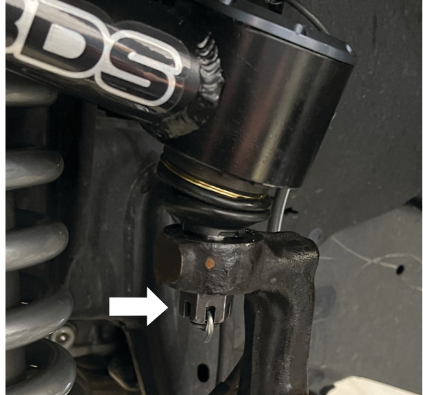
Fig. 6: Loosen upper control arm castle nut.
