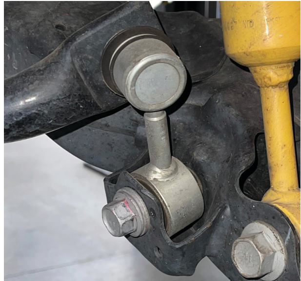
Fig. 2: Disconnect the sway bar end link.
