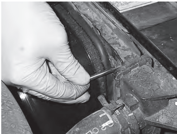
Install temp. probe near inlet hose...
