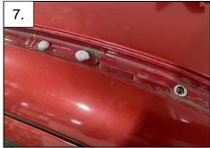
\*<u>NOTE:</u> two extra rivet nuts are included. A rivet nut installation tool can be purchased cheaply online if preferred\*
