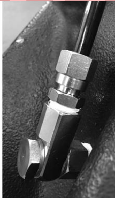
Figure 13. Air Locker bulkhead fitting assembly (170114)
