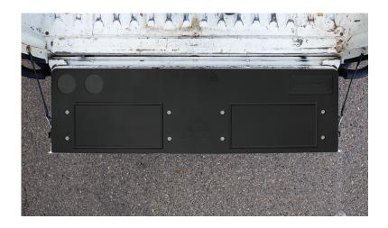
**1.** Remove the (8) screws holding the access panel to the tailgate. These screws will not be reused. **NOTE:** Do not remove the access panel after you remove the screws.
