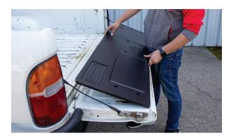
**3.** Install the supplied (8) washers and (8) Pozi dive screws to secure the tailgate table to the tailgate. Installing the screws may be easier if you initially start all thew screw, then tighten them. Be careful not to over tighten the screws and strip the plastic nuts in the tailgate.
