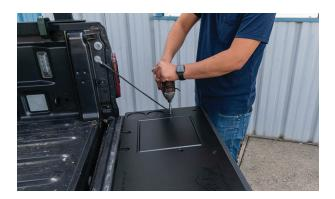
**4.** If desired, install the (4) supplied sheet metal screws into the pockets at the top of the tailgate table. These screws are meant to provide increased holding strength for the tailgate table but not necessary for most applications.
