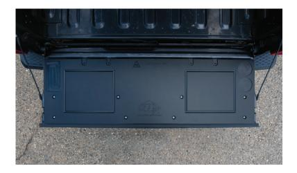
**1.** Remove the (8) screws holding the access panel to the tailgate. These screws will not be reused. **NOTE:** not remove the access panel after you remove the screws.
