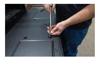
**4.** If desired, install the (4) supplied sheet metal screws into the pockets at the top of the tailgate table. These screws are meant to provide increased holding strength for the tailgate table but are not necessary for most applications.
