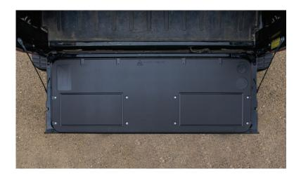
**1.** Remove the (8) screws holding the access panel to the tailgate. These screws will not be reused.
