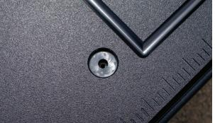
**3.** Install the supplied (8) Torx drive screws to secure the tailgate table to the tailgate. Installing the screws may be easier if you initially start all the screws, then tighten them. Be careful not to over tighten the screws and strip the plastic nuts in the tailgate.
