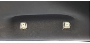
**4.** Position the rack on the interior of the roof and align the mounting slots in the rack with the plastic nuts in the roof. Use the provided hardware to mount the rack to the roof. Hand-tighten the mounting screws being careful not to strip the plastic nuts. If desired, place after-market grab handles over the mounting holes in the rack and reinstall the mounting bolts.
