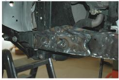
4. Bolt on the steering box with the hardware provided.
