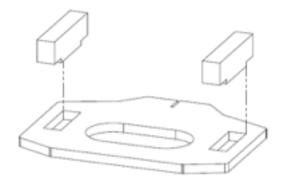
**12.** Flip the bracket over and plug weld the tabs to the bracket.
