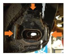
**5.** Disconnect the sway bar link, lower ball joint, & lower strut from the lower A-arm.
