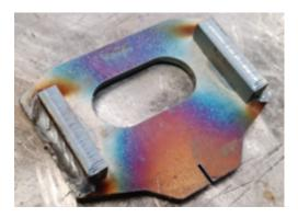
**13.** Grind the welds on the backside flush with the gusset using an angle grinder. Repeat Steps 10-12 for the remaining gussets.
