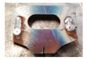
**14.** Align the slots onto the gussets with the slots on the frame. Tack weld the gussets to the frame.
