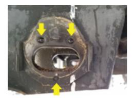
**9.** Using an angle grinder, grind the surface of the frame down to bare metal. The surface should be flat and free of paint.
