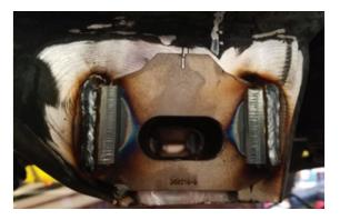
**11.** Weld the outer edges of the tabs.
