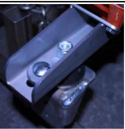
The mount can be assembled with the rubber mounts on the inner slot for a narrow frame or the outer slots for a widerframe. When the engine location is selected, tighten the carriage bolt to secures the mount location and then weld two 1/2" or more beads to secure the slide lock tab.
