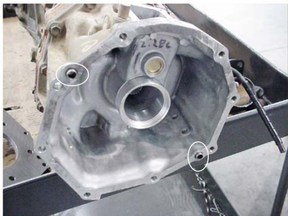
Make sure the dowel pins are in the stock tailhousing.
