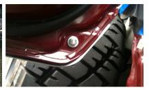
3. Next, install the lower door armor panel utilizing a 1" long screw, a flatwasher, and a nylock nut. Use the ½" long screws into the four square plastic inserts. Lightly tighten these screws to allow for a bit of alignment adjustability before final tightening.
