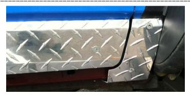
5. Proceed with installing the rocker armor. Line up the tabs in the rocker with the oblong holes in the FJ's body. Insert the tabs and push the rocker piece forward until tabs fully engage within the oblong holes.
