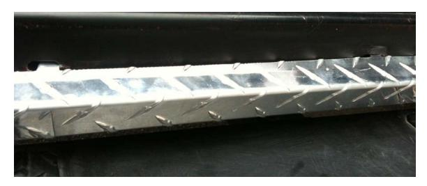
6. Once all the tabs are fully engaged, you should now be able to thread a ½" long screw into the square plastic insert at the rearward end of the rocker armor piece. Next, push in on the rearward end of the rocker armor piece towards the FJ's body until you can access the wheel well square plastic insert through the mounting tab on the rocker
