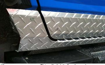
armor. This will slightly flex the rocker armor so that it can conform to the curve of the FJ's body.
