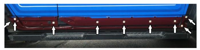
2. Begin the install with the rear access door panel. The rearward hole utilizes a 1" long screw, a rubber snubber, a flatwasher, and a nylock nut. Place the screw through the hole and capture the snubber on the inner side, then set the threads through the hole on the door. You'll need a slight amount of alignment adjustability before the final tightening, so only lightly tighten this nut at the moment. Now thread a ½" long screw into the forward hole and lightly tighten.
