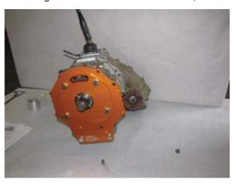
**STEP 41**Install provided coupler to transmission
