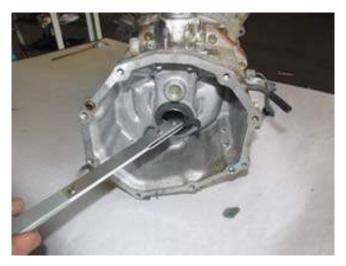
**STEP 40**Install Seal housing with seal with a rubber
