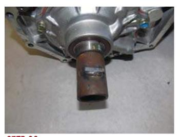
**STEP 38**Install 2 M8-1.25 studs on to the transfer case with blue Loctite in the locations shown
