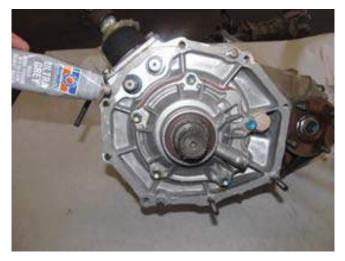
**STEP 40**Remove stock seal from back of transmission
