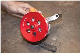
**STEP 9** - INSERT BOLT WITH SPACER
