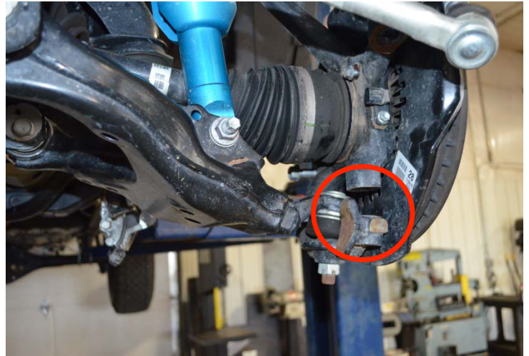
Two bolts removed from spindle, LCA is no longer attached to spindle.
