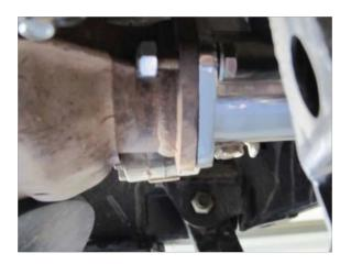
**STEP 16** Install the O2 Sensor/EGR Gasket onto the down pipe.
