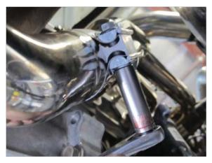
**STEP 17** Install the O2 Sensor onto the down pipe.
