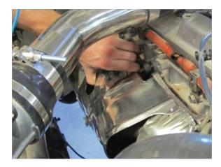
**STEP 3** Unbolt the stock down tube from the catalytic converter.
